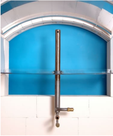
Fig.3 Compressed air baffle, installed in the port bottom
